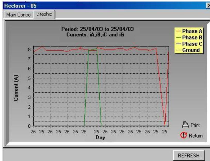
Fig. 4 – The on line currents logging.
