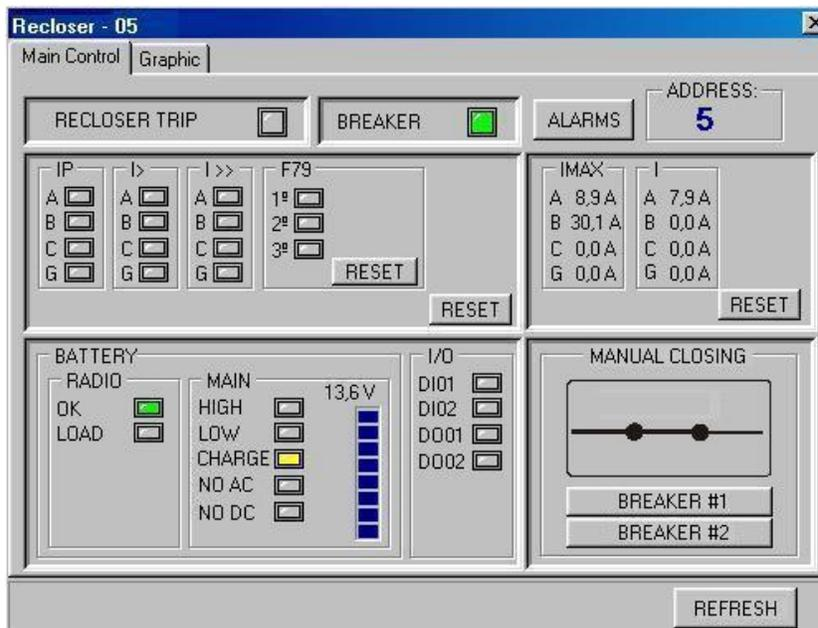
Fig. 5 – The main control recloser window.
