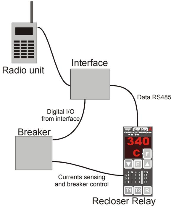
Fig.6 – The Remote Unit block diagram.
