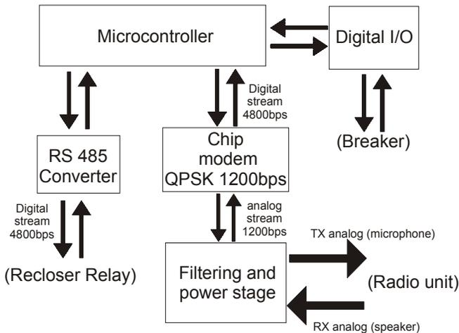
Fig.7 – Details of interface
