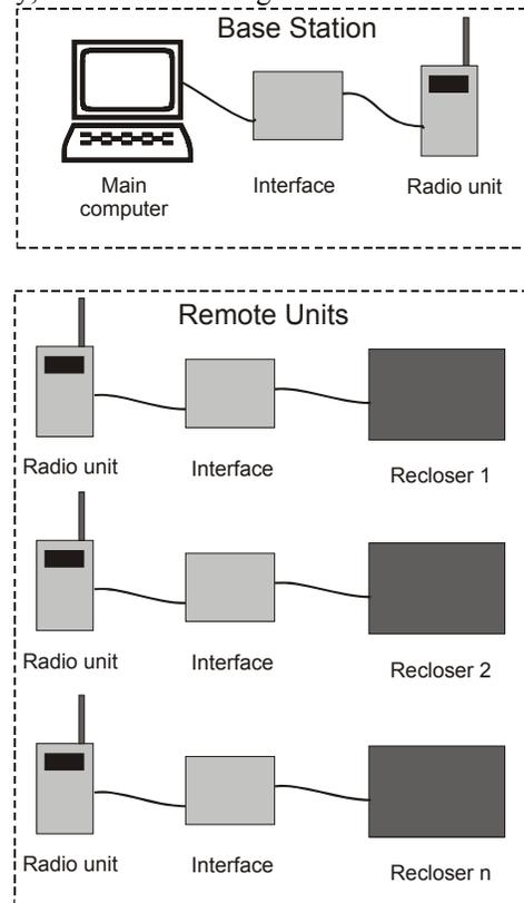
Fig.1 – Monitoring system based on radio control
